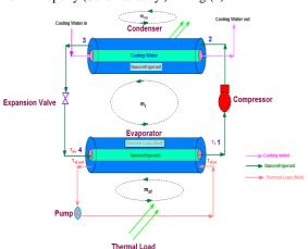
**Fig: 2.** Schematic Diagram of Vapour Compression Refrigeration System Model
