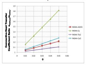
Fig: 10. Variation of Convective heat transfer coefficient ratio with volume fraction (φ) of R134a using different nanoparticles
