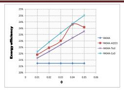
Fig: 22. Variation of Exergy Efficiency with volume fraction (φ) of VCRS with R404A using different nanoparticles
