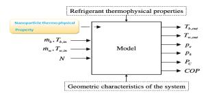
Fig: 1. Vapour Compression Refrigeration System Model
