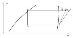
Fig: 3. Vapor Compression Cycle
