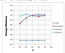
Fig: 20. Variation of Exergy Efficiency with volume fraction (φ) of VCRS with R134a using different nanoparticles
