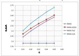
**Fig: 16.** Variation of C.O.P with volume fraction (φ) of VCRS with R404A using different nanoparticles
