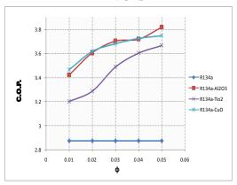
**Fig: 14.** Variation of C.O.P with volume fraction (φ) of VCRS with R134a using different nanoparticles
