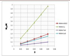
**Fig: 8.** Variation of Thermal conductivity Ratio with volume fraction  $(\phi)$  of R404A using different nanoparticles
