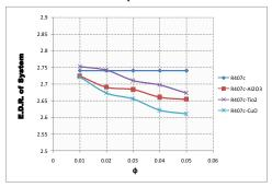
Fig: 18. Variation of Exergy Destruction ratio with volume fraction (φ) of VCRS with R407c using different nanoparticles
