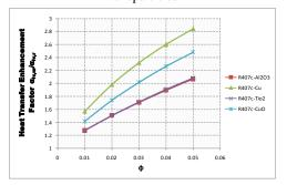
Fig: 13. Variation of Heat transfer Enhancement Factor with volume fraction (φ) of R407c using different nanoparticles
