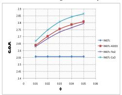
Fig: 15. Variation of C.O.P with volume fraction  $(\phi)$  of VCRS with R407c using different nanoparticles
