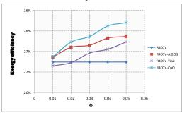
Fig: 21. Variation of Exergy Efficiency with volume fraction (φ) of VCRS with R407c using different nanoparticles
