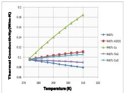
**Fig: 5.** Variation of Thermal conductivity with Temperature of R407c using different nanoparticles
