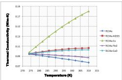
**Fig: 6.** Variation of Thermal conductivity with Temperature of R134a using different nanoparticles
