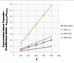
Fig: 9. Variation of Convective heat transfer coefficient ratio with volume fraction ( $\phi$ ) of R407c using different nanoparticles
