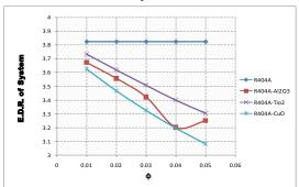
Fig: 19. Variation of Exergy destruction ratio with volume fraction (φ) of VCRS with R404a using different nanoparticles
